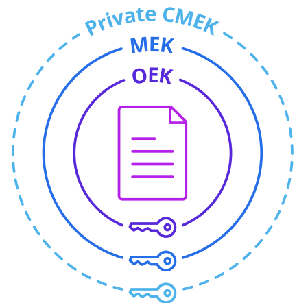
The document is encrypted by the OEK, which is then wrapped by the MEK. If CMEK is active, the MEK is wrapped by the CMEK adding a third layer of encryption to the document.
